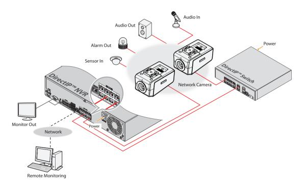
DirectIP<sup>™</sup> NVR makes it easy to use cameras without extra network configurations. Each camera can be controlled via the DirectIP<sup>™</sup> NVR setup menu, without any PC. For detailed camera settings, please see the camera setting pages of DirectIP<sup>™</sup> NVR manual.
